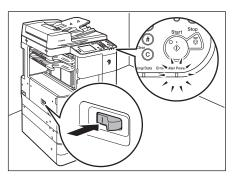
Press the main power switch (located on the left side of the machine) to the "I" side.
